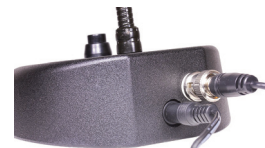
PULSE base accepts a user-supplied voltage input
