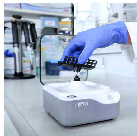
Quickly mount rotors by pushing the rotor onto the drive shaft until it clicks. Remove easily by pulling straight up.
